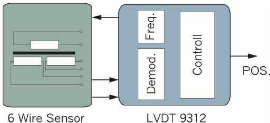
The LVDT9312 accepts a wide voltage supply range from 9V to 36V and provides galvanic isolation between the cRIO and the demodulator interface. The module is useable within the NI cRIO real time environment and can also be plugged into a NI R-series expansion chassis with PCI / PXI FPGA card. We provide all drivers required for the cRIO system and LabVIEW integration examples.
