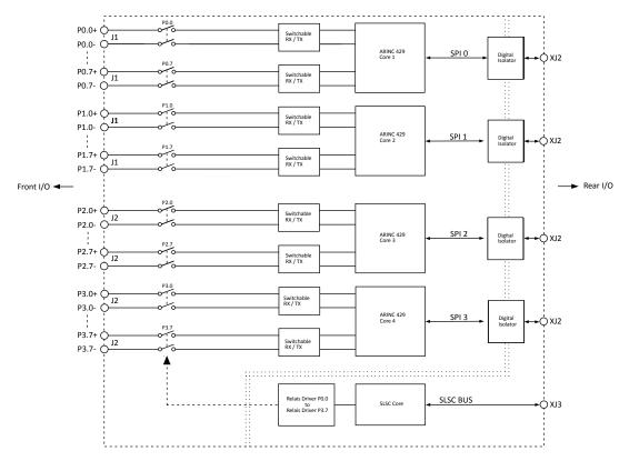
**Note** Diagram only shows one channel per front connector J1.
