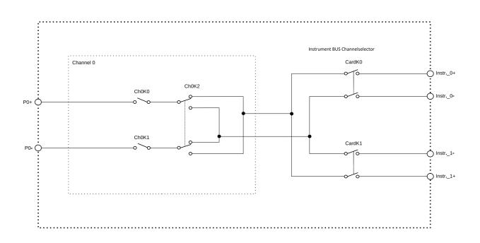
**Note** Diagram only shows one out of 16 channels. Per daughter module one instrument bus can be selected.
