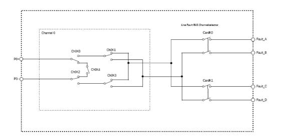
Note Diagram only shows one out of 16 channels. Per daughter module one line fault Bus can be selected.
