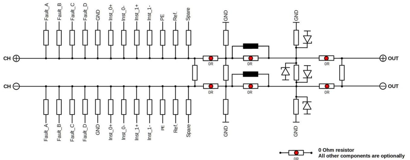
**Note** Diagram only shows one channel. All components without a labeling, are optional.
